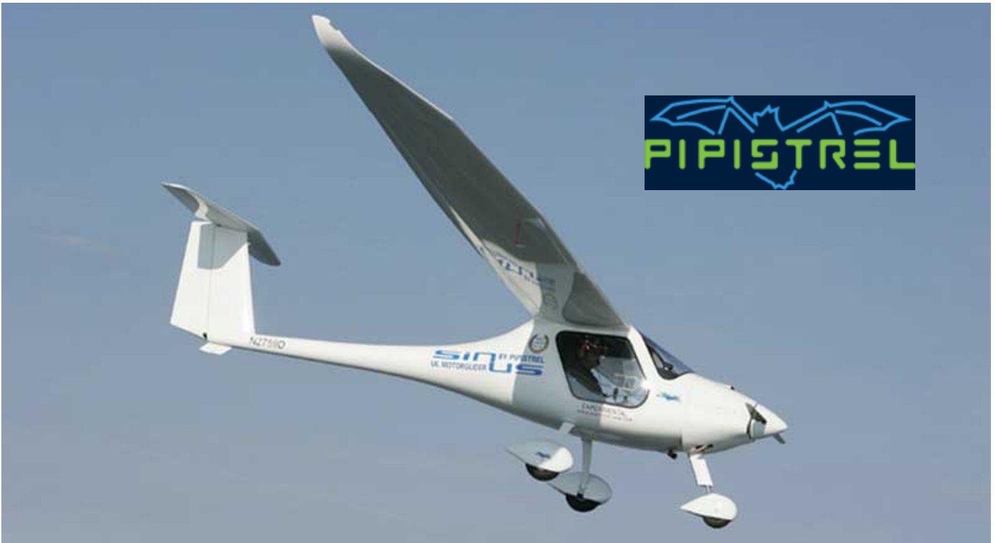
The Pipistrel Sinus can be configured either with a nose wheel or as a tail-dragger.
